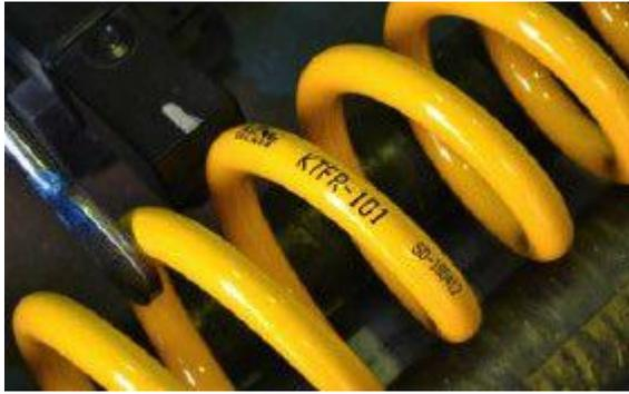
Once powder coated the coil is then Ink Jet printed with durable, fast curing ink with both part number and batch number for traceability.
