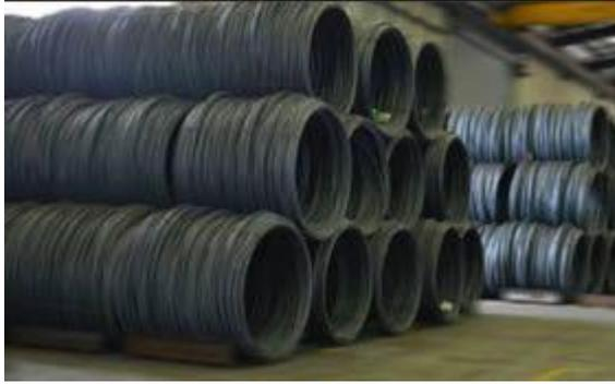
Only X5K material is used. X5K is a new generation High Strength Spring Steel which with-stands higher operating stresses and has superior resistance to sag, improved toughness and improved corrosion fatigue properties.
