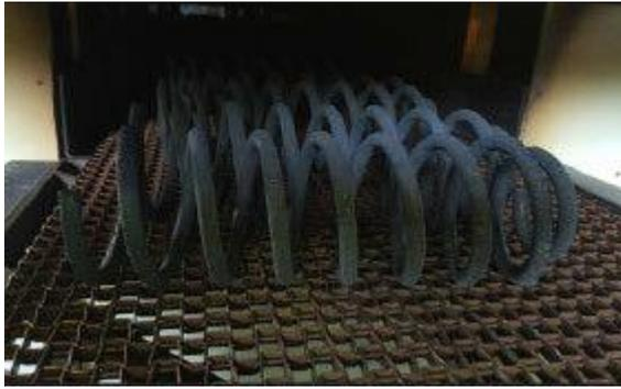
After the Hardening process the coil is then placed into the Tempering oven and heated back up to 400 degrees Celsius . Coil will be now tempered to a 54 HRC. This is done via a computer controlled and monitored gas furnace.
