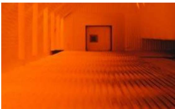
Gas furnaces are used for their extremely clean and efficient heating properties. Coils are heated to around 1000 degrees Celsius before being rolled.
