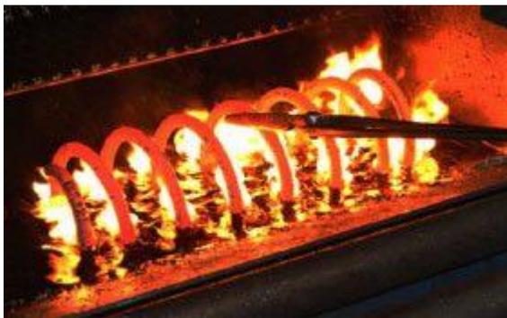
Once the coil is rolled it is then placed into the Quenching oil whilst still at 850 degrees Celsius and hardened to 62 HRC (Rockwell hardness)
