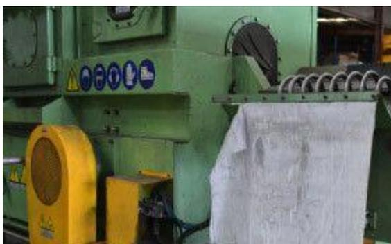
The coil is now placed into our Conveyor fed shot peener and rotated for 100% coverage. This gives the coil a high intensity finish to ensure maximum fatigue life and an optimal surface for the powder coat to be applied to.
